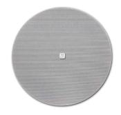
The versatile CMX20DT 8" two-way built-in loudspeaker produces a deep and warm sound ideal for speech and music. When using the loudspeaker at 16 ohms, you can connect up to 4 loudspeakers in parallel on each channel of a standard 4 ohms amplifier.
