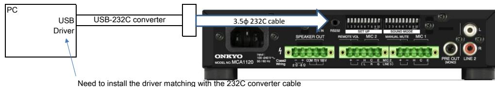
Example of the cabl USB-232C converter cable
